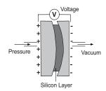
This digital manometer achieves stable, quick responding, repeatable and precise measurements by using an advanced piezo-resistive sensor. Integrating the sensor and circuits together allows a tighter accuracy specification based on the reading value instead of the full scale value. The Piezo-Resistive sensor is a diaphragm formed on a silicon subtrate, which bends with applied pressure and generates millivoltage or millicurrent proportional to the pressure applied.
